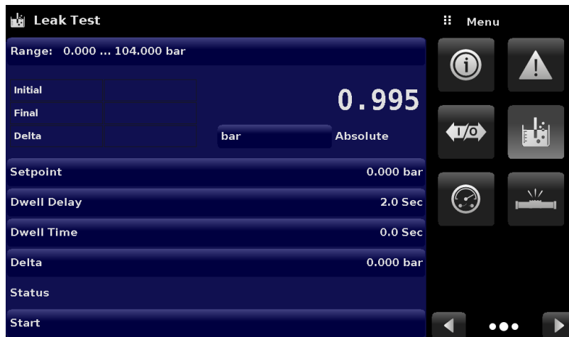
Figure 6.4.12 Leak Test App
