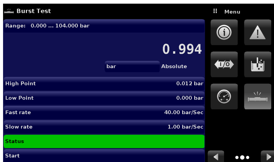
Figure 6.4.14-B Burst Test Complete (No Burst)
