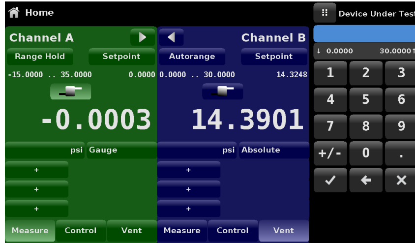
Figure 8.9.2.3-C - DUT pressure for purge sequence
