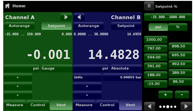
Figure 6.4.1.2.3-B - DUT Pressure Value Entry
