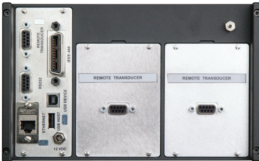
Figure 5.4 B - Two remote transducer interface connections installed
