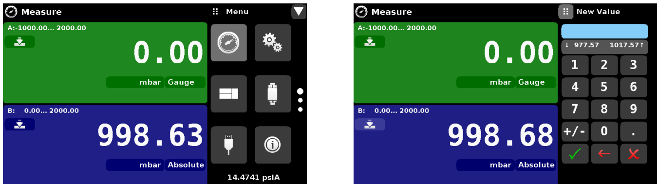
Figure 6.4.1.3 - Zero Button, Gauge - Absolute
